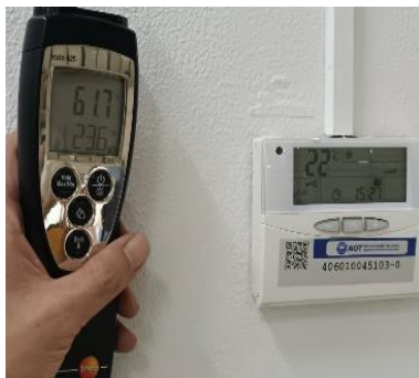
2 nd Floor Temperature and Set Point
